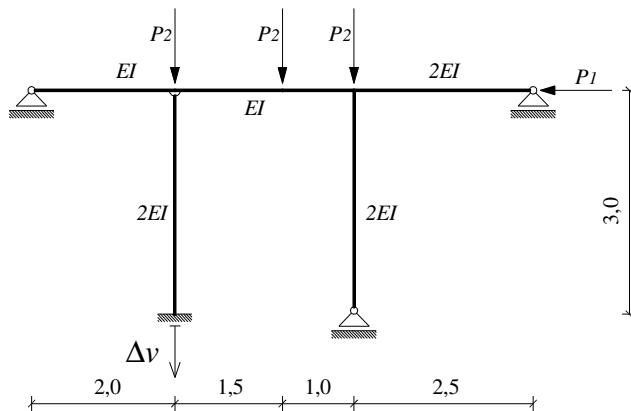
$$\begin{aligned}\Delta v &= 1\text{cm} \\ E &= 3 \cdot 10^7 \text{ kN/m}^2 \\ b/h &= 35/40[\text{cm}] \\ P_1 &= 120\text{kN} \\ P_2 &= 140\text{kN}\end{aligned}$$
