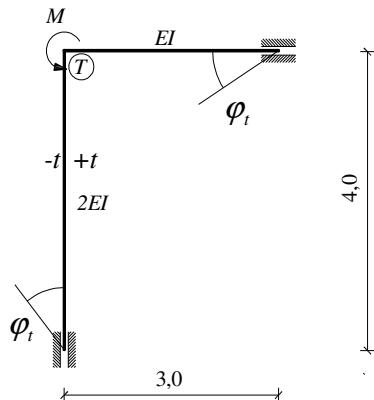
$$\begin{aligned}\pm t &= 13^\circ C \\ \alpha_t &= 10^{-5} K^{-1} \\ E &= 3 \cdot 10^7 \text{ kN/m}^2 \\ b/h &= 30/45[\text{cm}] \\ M &= 174\text{kNm} \\ \varphi_t &= 0.004\end{aligned}$$
