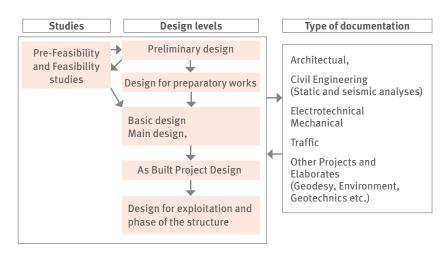
Figure 2: Main levels of design and type of documentation according to the Law on Construction
