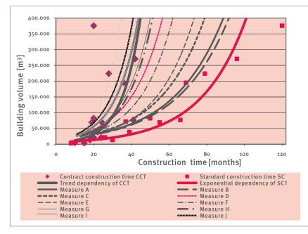
Figure 3. Impacts of the measures for construction time shortening in multifunctional buildings segment
