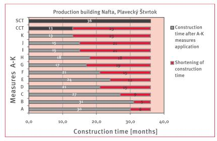
Figure 5. Impacts of the measures applied at Production building Nafta, Plavecký Štvrtok
